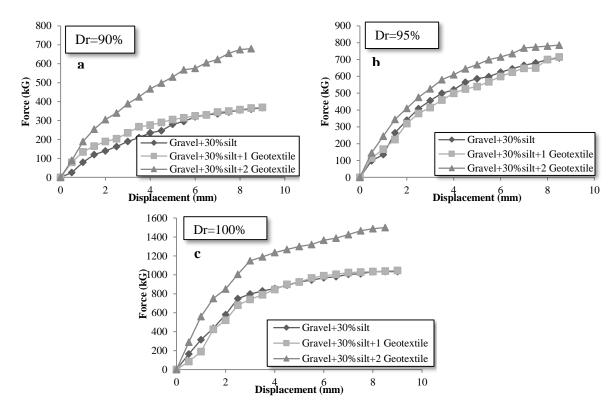
Figure 8. Comparison of gravel+30% silt bearing capacity in reinforced and unreinforced position in several relative densities (Sadeghi et al., 2010)
