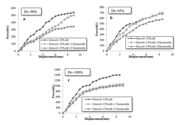
**Figure 7.** Comparison of gravel+15% silt bearing capacity in reinforced and unreinforced position in several relative densities (Sadeghi azar et al., 2010)
