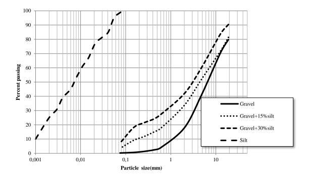
Figure 1. Grain size distribution for soils used in this study (Sadeghi azar et al., 2010).
