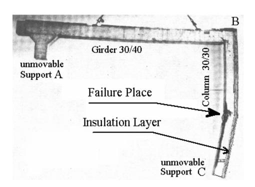
Fig. 3.6: Collapse of frame work No. 4 in case of ISO-Fire
