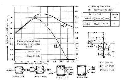
Fig. 3.2: Development of the calculated corner moments of the frame-work in case of fire
