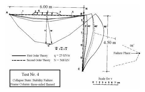
Fig. 3.5: Calculated deformation of Frame Work No. 4 in case of ISO-Fire
