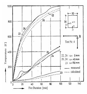
Fig. 3.1: Measured and calculated temperatures in case of ISO834-Fire
