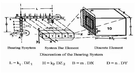
Fig. 2.1: Axial and cross-sectional discretisation of a bearing system in case of fire
