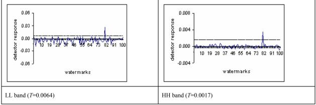
Figure 3. Detector response for unattacked watermarked I Frame
