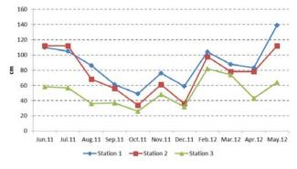
Figure 3. Monthly variation of Secchi disc depths in three stations.
